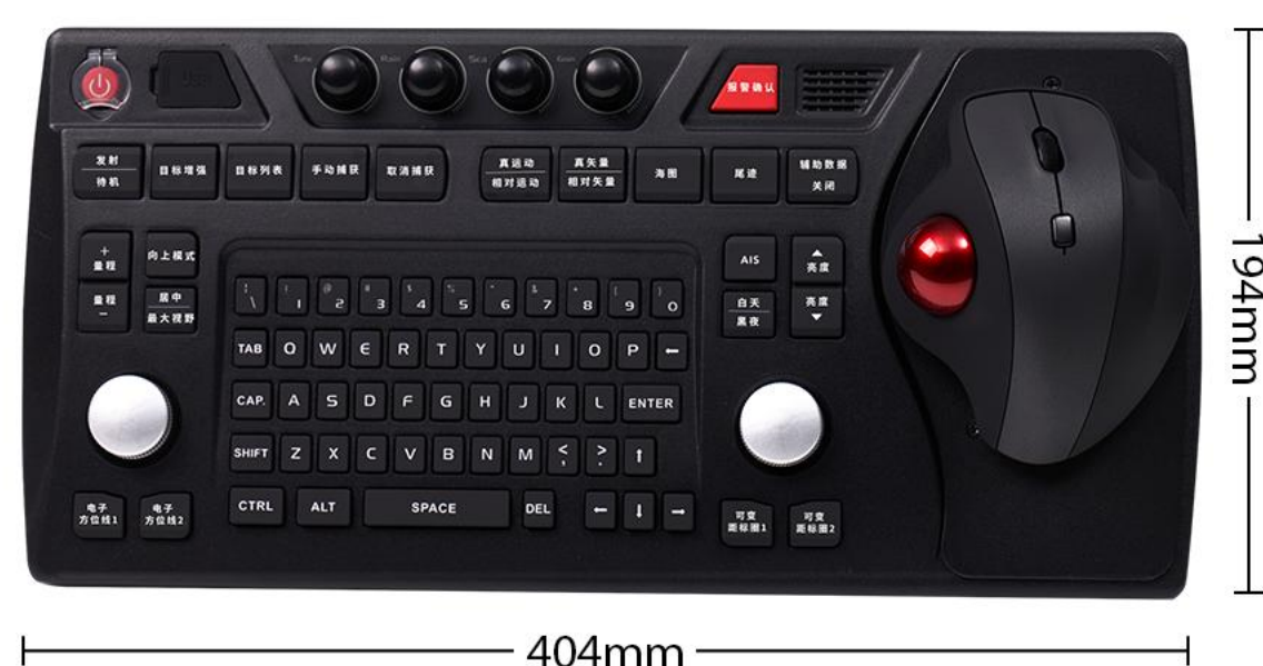
[Human-machine Interaction Unit HLD-IU600 3kg]
