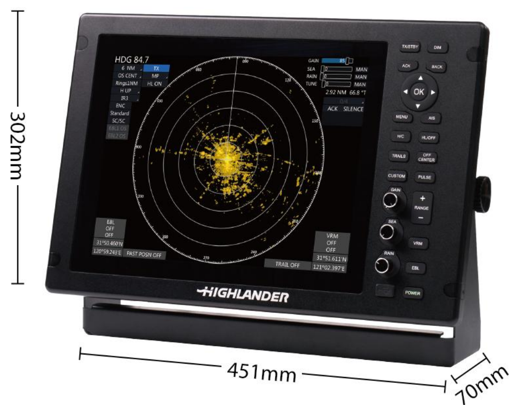
[On-board all-in-one machine HLD-MCS215]
