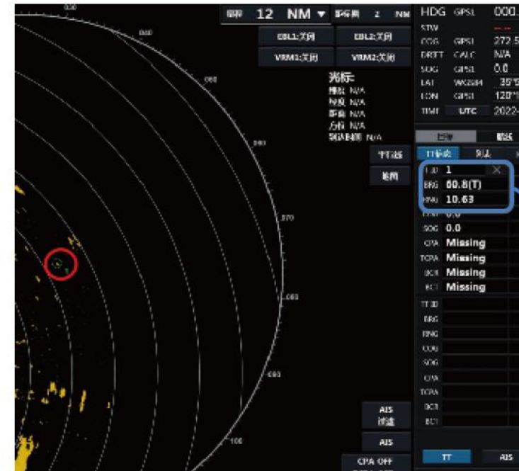
Detection range of a standard 10m 2 sphere at X-band (IMO standard 4.9NM)
